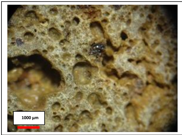
Figure-13: The open pores produced by bloating of the raw materials mixed with motors waste oil.
