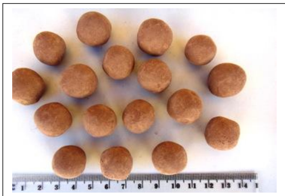
Figure-3: Pellets molded by hand for lightweight Aggregate preparation (before firing).
